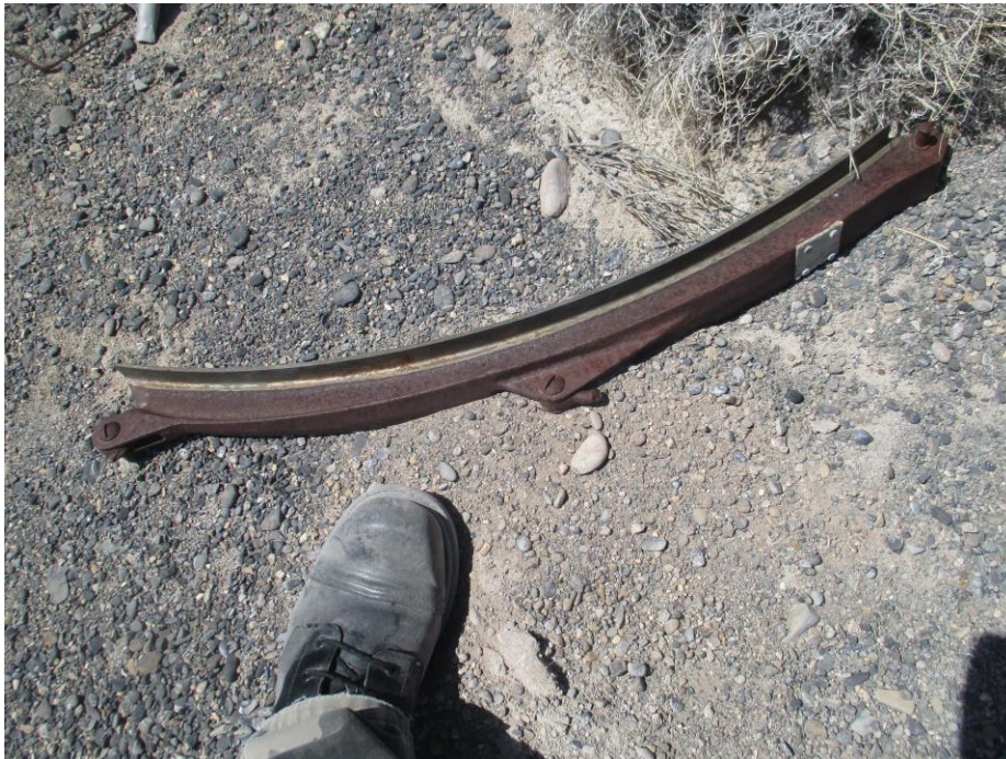
Part of a wing flap mechanism
