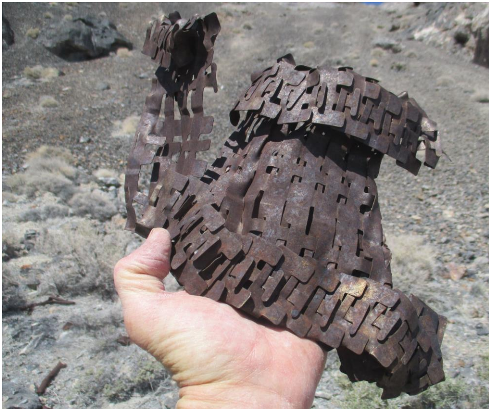
Part of a flexible chute for .50 cal machine gun ammunition
