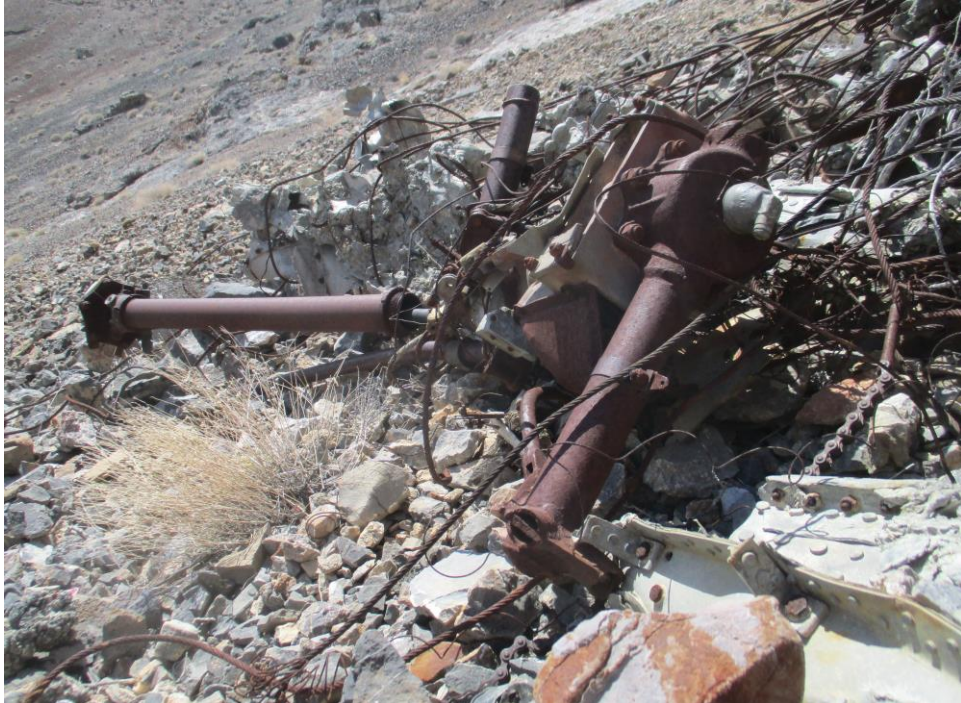
The ball turret support and drive mechanism
