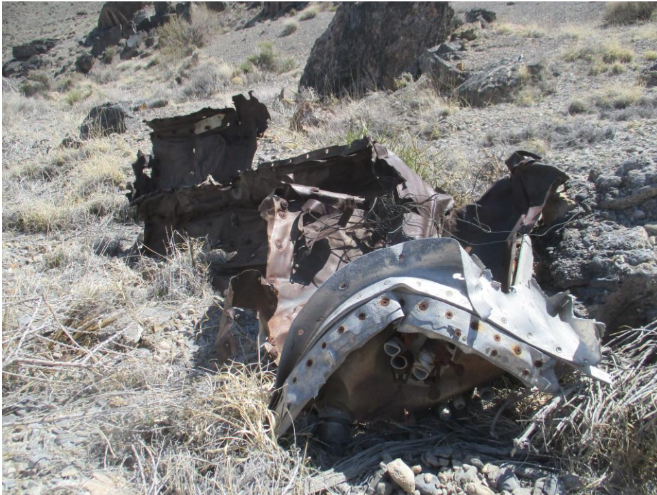
Part of a stainless steel firewall for a Pratt & Whitney R-1830 engine
