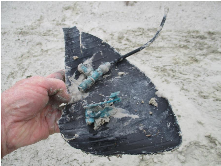
A small aluminum linkage and a fluid junction block resting on rubber from a landing gear inner tube
