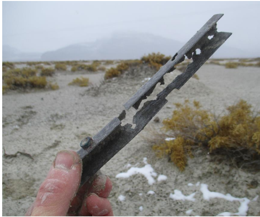
This piece of aluminum stringer shows how badly the parts have corroded
