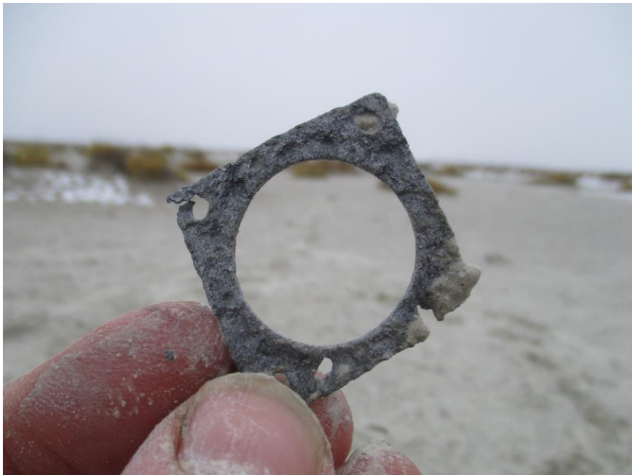
A small bezel from the instrument panel, probably for a switch or button
