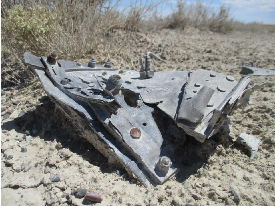
The multiple layers of riveted heavy-duty aluminum suggest this piece was from a wing root
