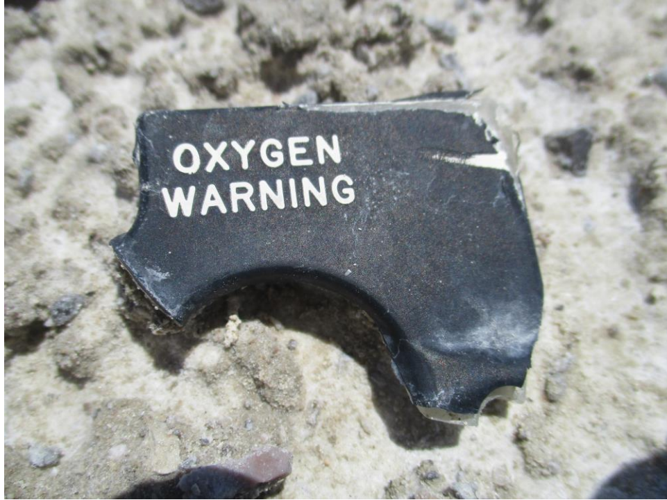
Part of a low oxygen placard located next to a warning light in the cockpit
