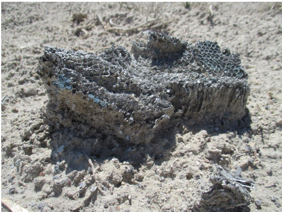
Aluminum honeycomb material used in the horizontal stabilizer of the F-100
