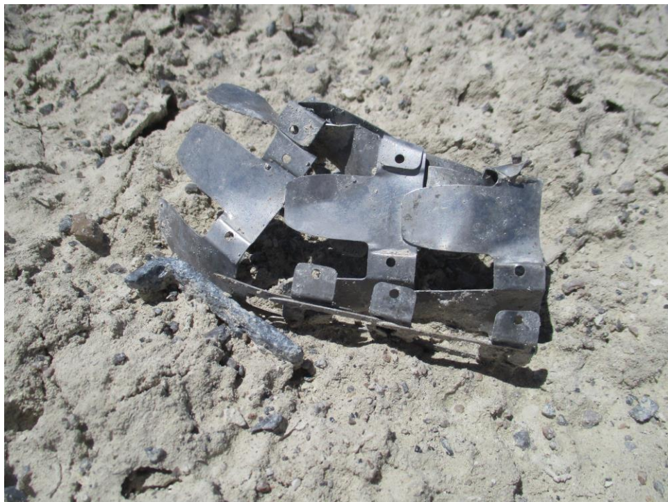
Part of an ammunition chute from a 20 mm cannon
