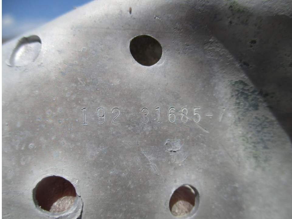
The "192" part number prefix confirms the wreckage is from an F-100
