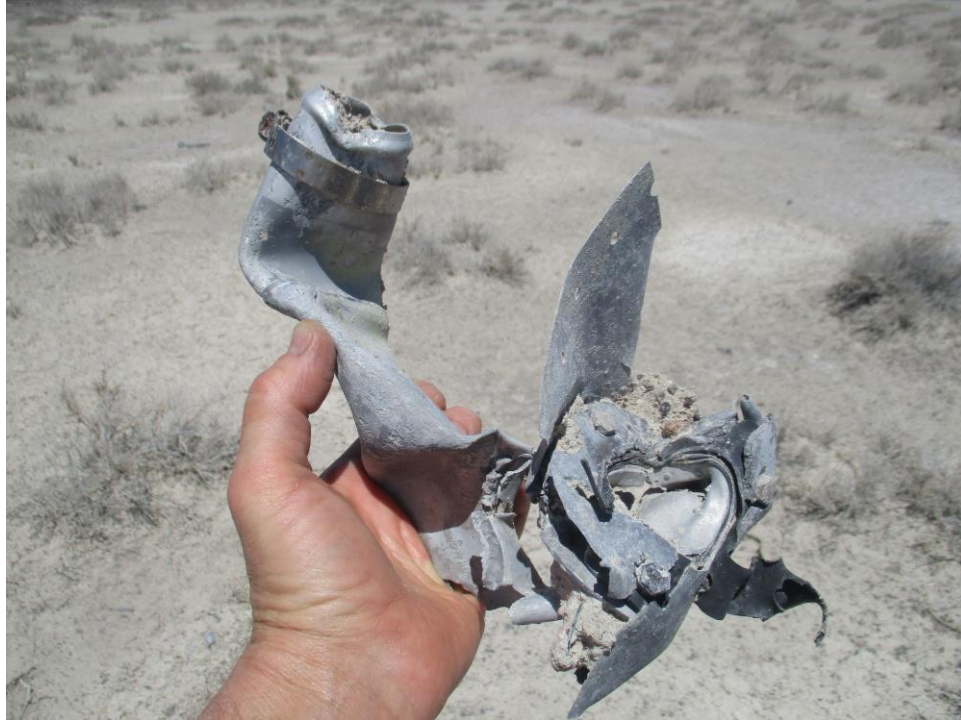
Part of an aluminum air conditioning pipe from the cockpit
