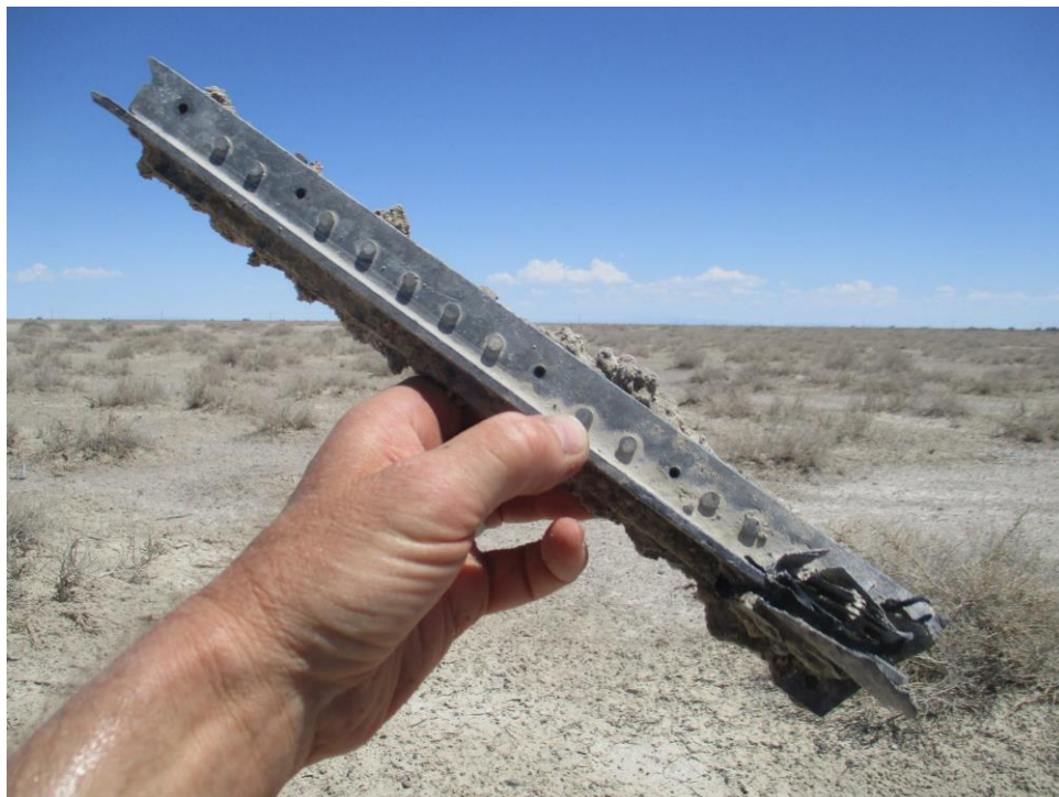
Many rivets are visible on this aluminum stringer
