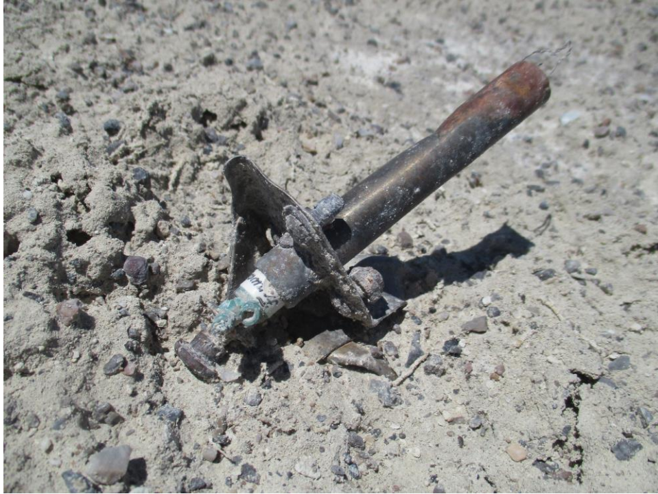
An engine igniter
