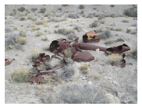
The warhead section is in the center, with the rear fuselage to the right and fuel tank above
