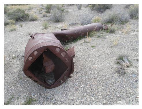
The intake of the pulse-jet engine, with intake shutters and fuel injectors missing
