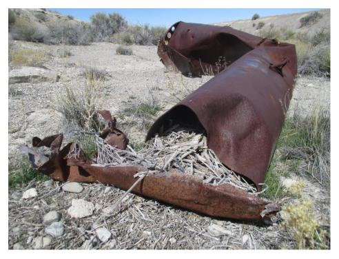
The tailpipe of the pulse-jet engine, which bent in half on impact
