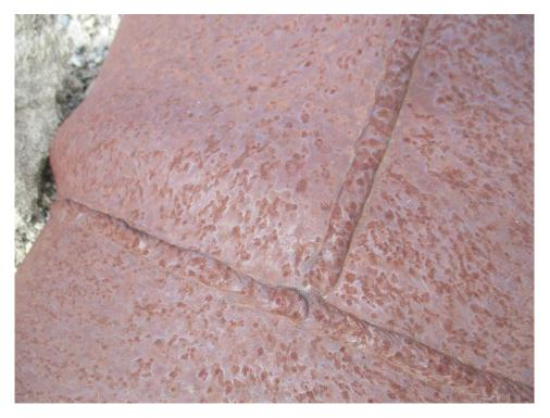
An example of the welded steel construction of the fuselage
