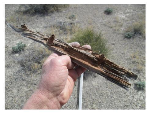
The aviation-type fasteners in this wood mean it was part of a wing
