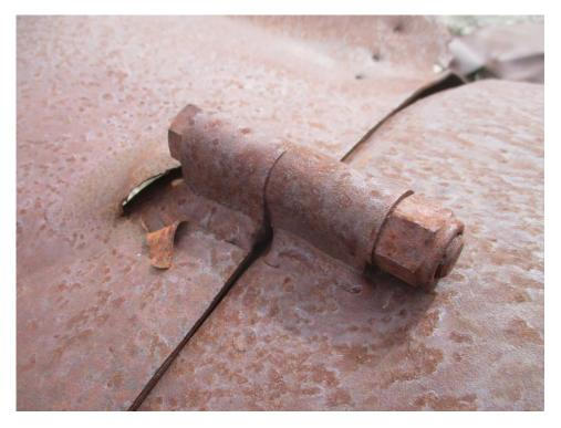
Large exterior bolts held the warhead to the fuel tank section
