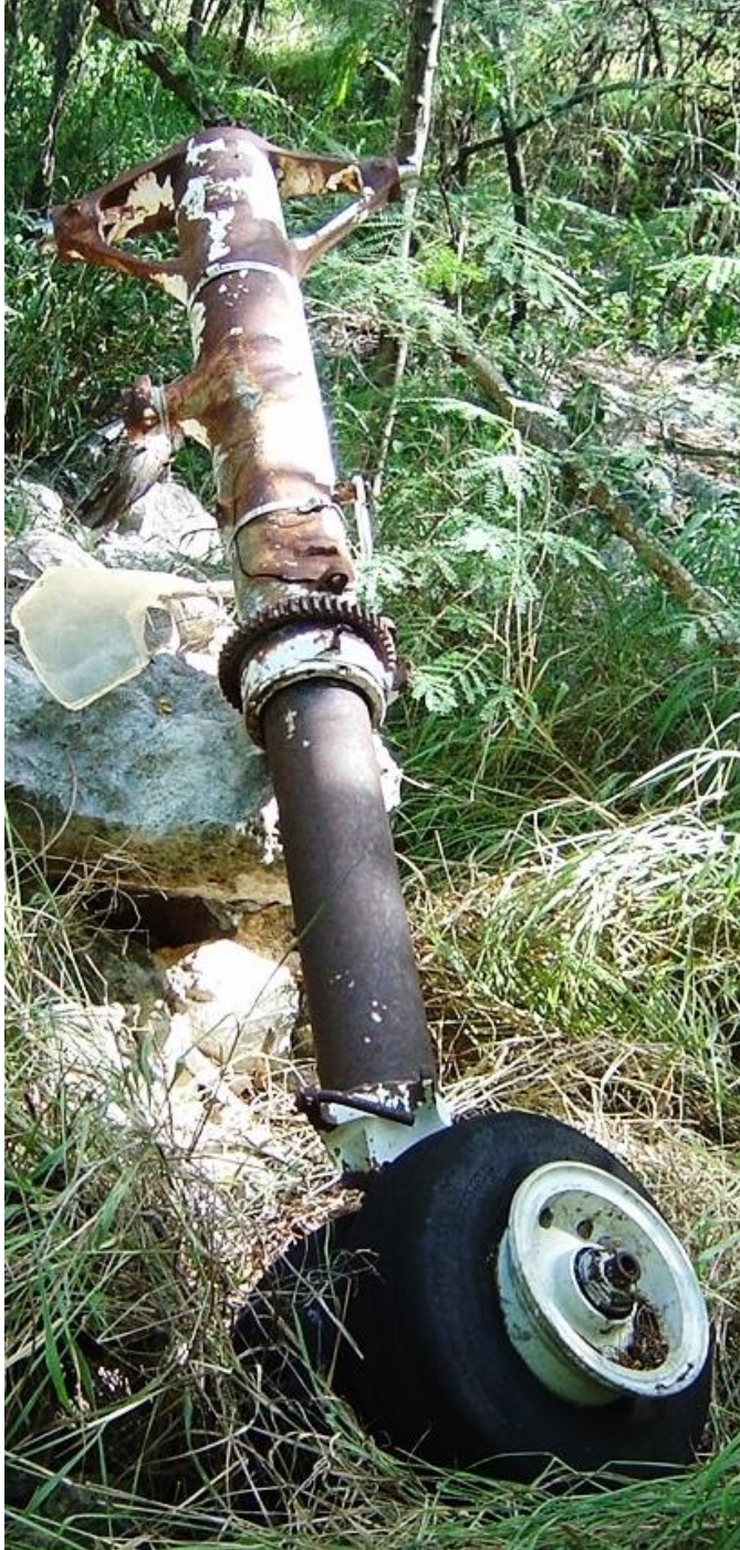
Front nose landing gear, the pilot may have tried to steer this or it may have malfunctioned, photos circa 2004 and 2007
