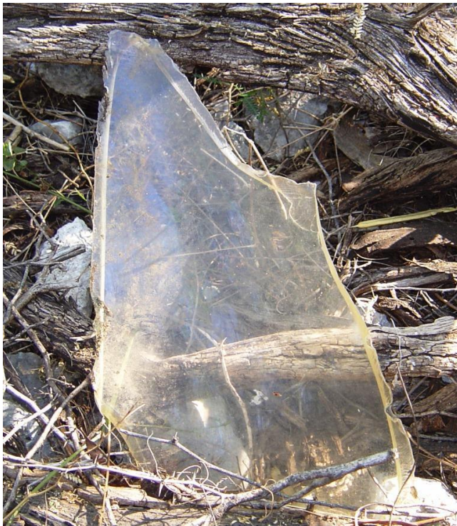
Large piece of Plexiglas from the canopy, many pieces of it littered the site from when the crew attempted ejection, photo circa 2007
