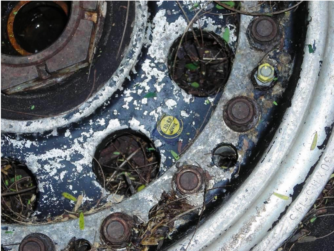
Close up of the main landing gear wheel rim has sticker with last overhaul date of 10/69 on it, photo circa 2007
