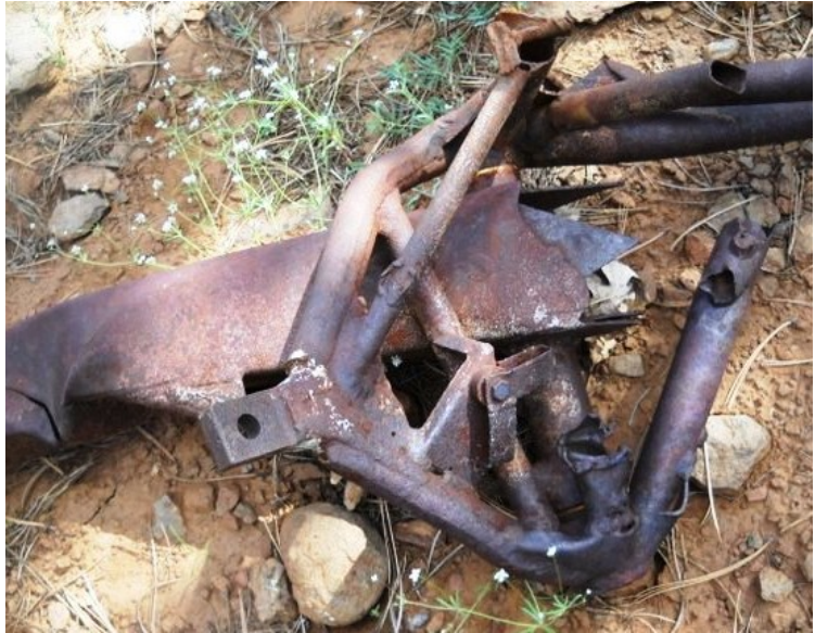
Landing gear leg with wing strut mount
