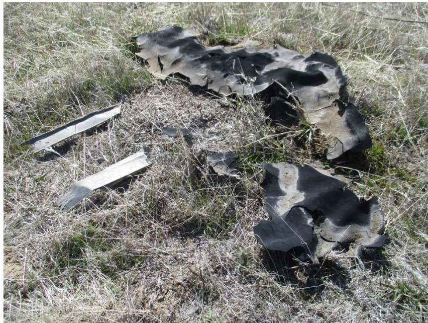
Melted rubber, probably from a self-sealing fuel tank
