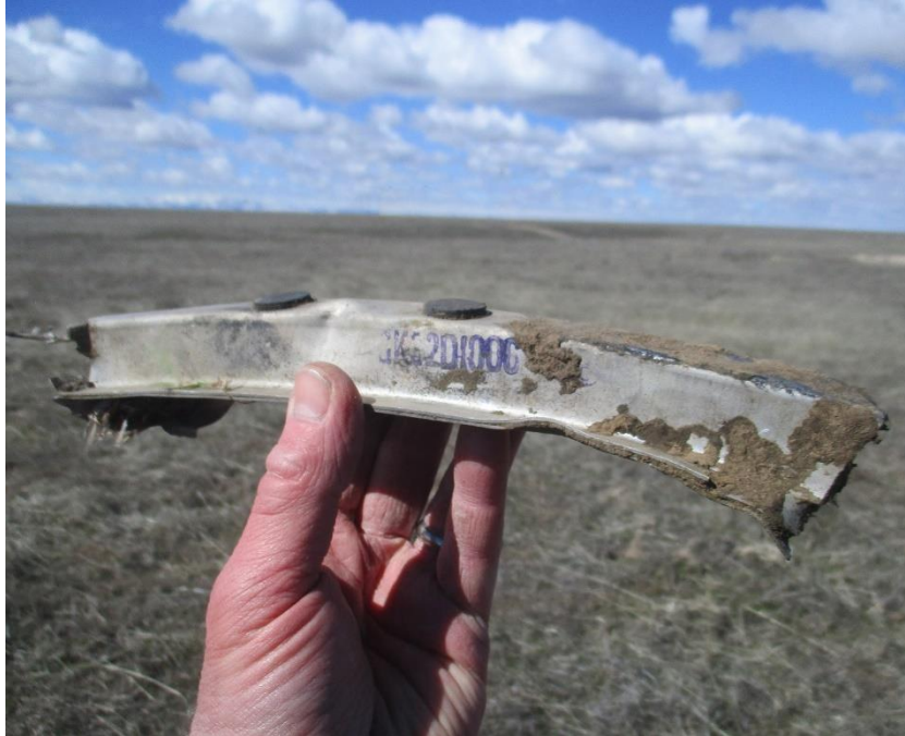
A part number stamped in ink. "GK" indicates this piece was made at the General Motors plant at Kansas City, KS
