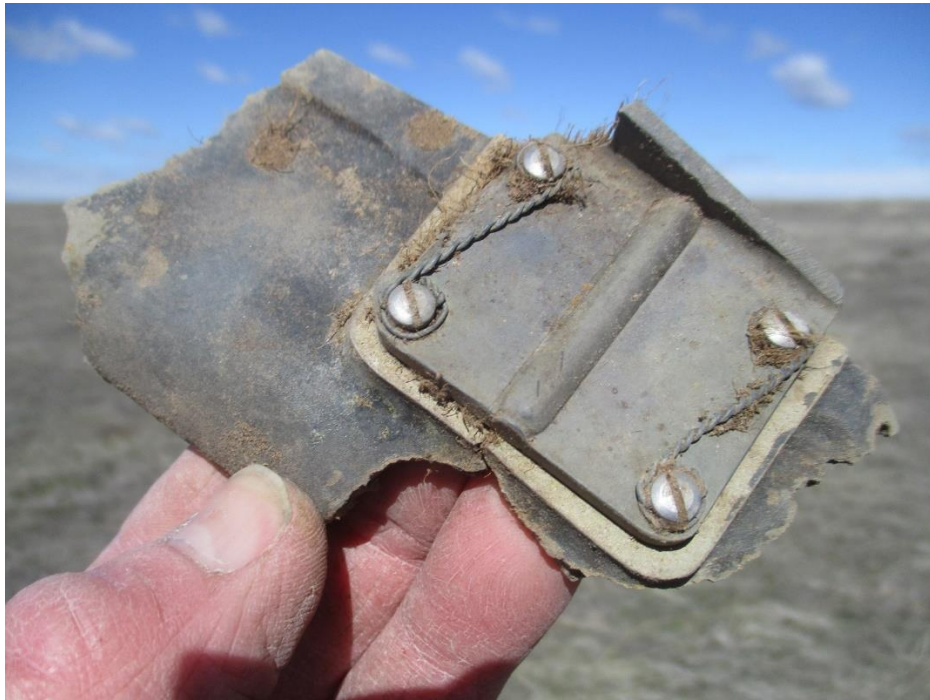
The safety wire on this piece is still intact after impacting the ground 76 years ago
