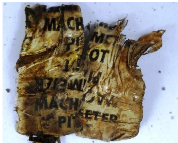
Machmeter label from pilot tube line
