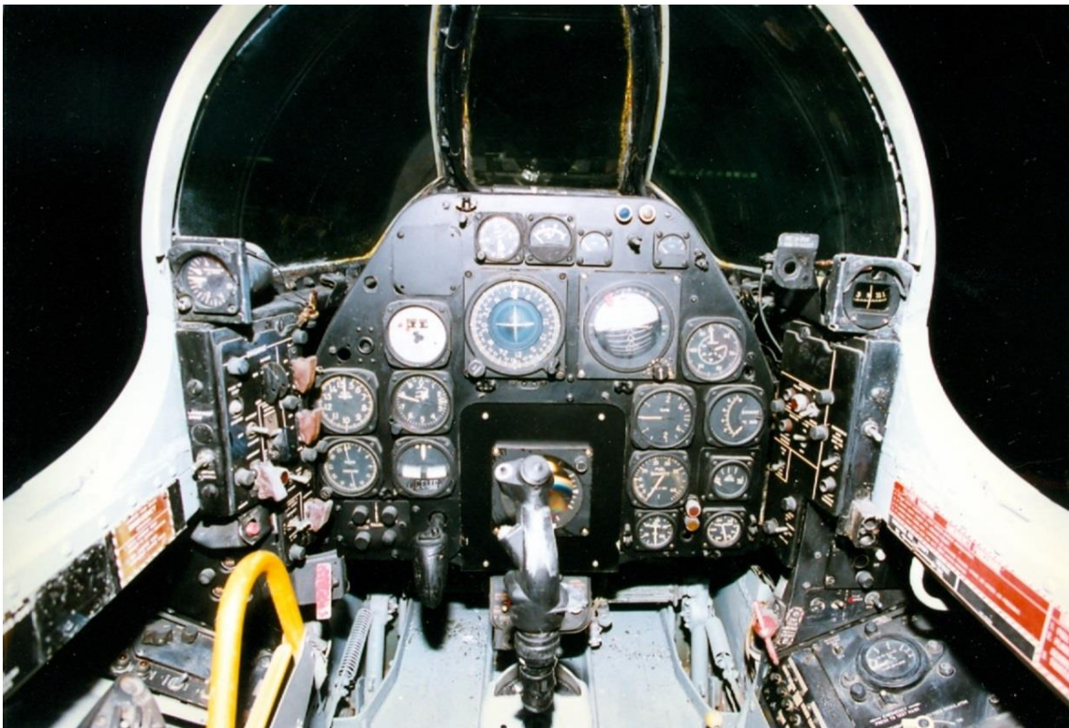
F-86D cockpit, note radio controls require looking down and to the side
