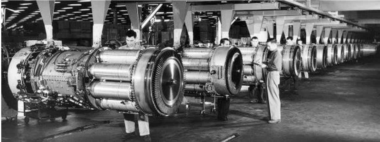
Production of the J47 engine at the GE Aviation Lockland, Ohio plant, circa 1950
