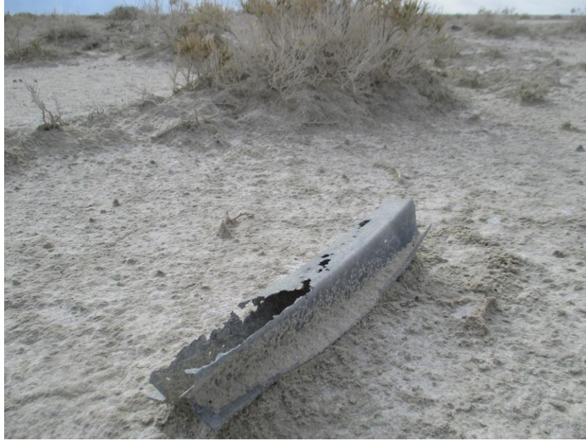
Badly corroded aluminum stringer on the salt flats
