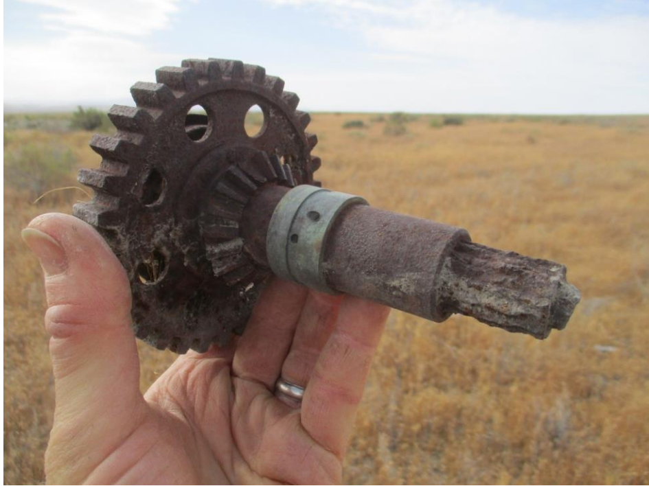
Gear, bearing, and splined shaft from engine
